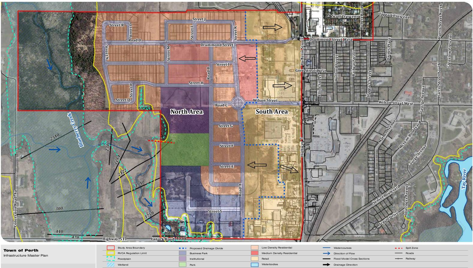
**Proposed Conditions Stormwater Drainage**
